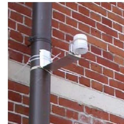
Measurements of nitrogen oxides with passive samplers
