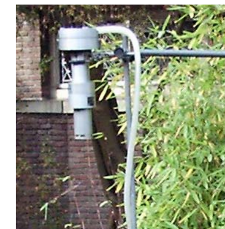
Measurement of fine particles with pump and sampling head
